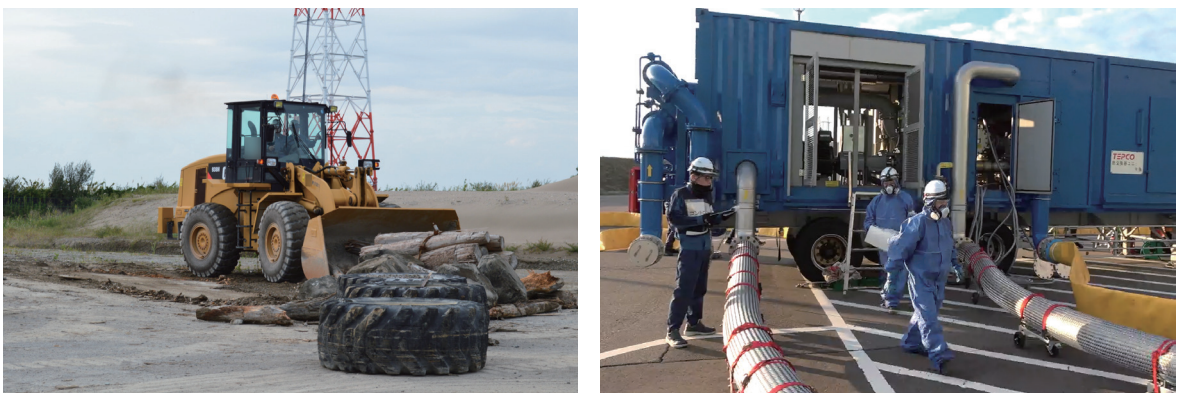
Regular training and drill on the operation and connection of mobile equipment, such as the removal of rubble with wheel loaders (left) and connecting alternative heat exchanger trucks (right), etc., is carried out to ensure that this equipment can be quickly and correctly used in times of emergency.
